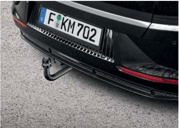
Tow bar, detachable. Whenever you have substantial cargo in tow, this top-quality, corrosion-resistant steel tow bar is ideal for efficient transportation.
